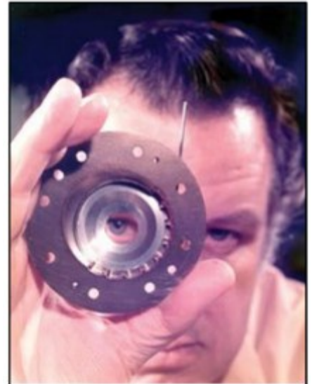
Diamond window from the Pioneer Venus Mission spacecraft (Photo Hughes SCG Heritage).
