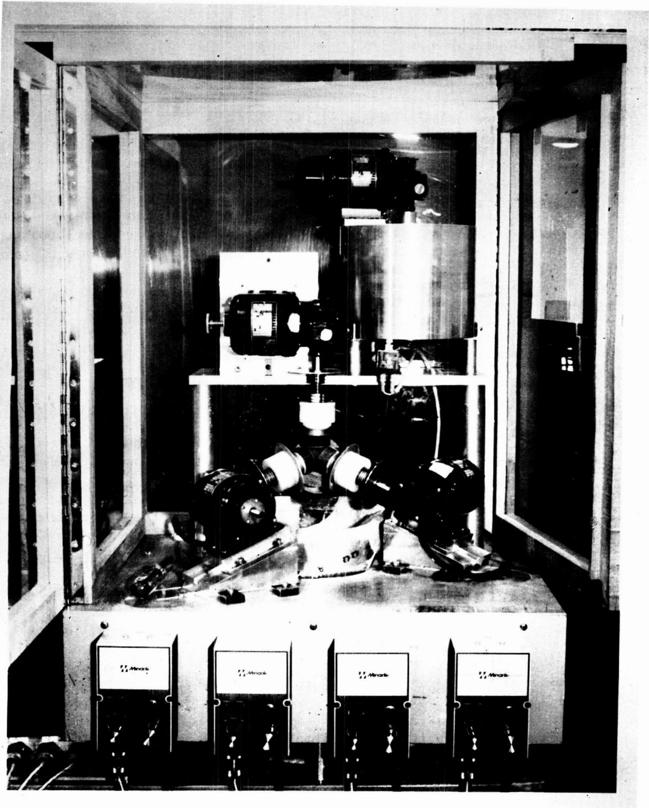
Figure 6. Polishing machine with enclosure.
